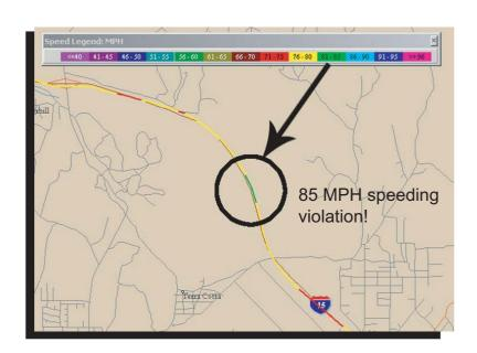
The route line is color coded to indicate the speed the vehicle was traveling. The color on the route line corresponds to the Speed Legend toolbar.
